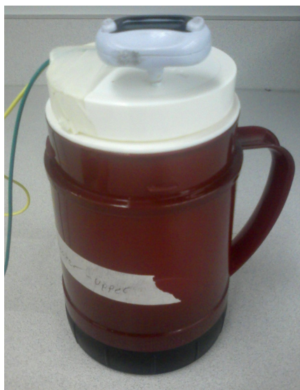
Illustration 2: The coffee-cup calorimeter used in this experiment
