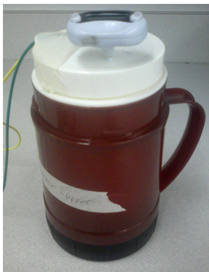
Illustration 2: The coffee-cup calorimeter used in this experiment
