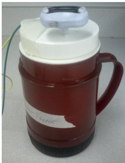
Illustration 2: The coffee-cup calorimeter used in this experiment
