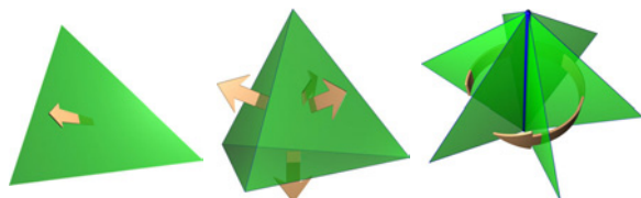
Figure 4: Discrete Physical Quantities: in our geometric discretization, fluid flux lives on faces (left), divergence lives on tets (middle), and vorticity lives on edges (right).
