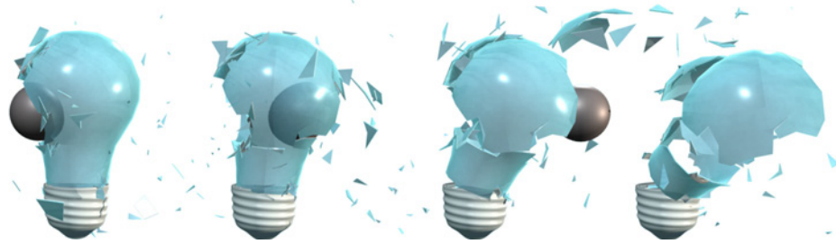
Figure 1: A measure of discrete strain is used to fracture a thin shell in this simulation of a shattering lightbulb.
